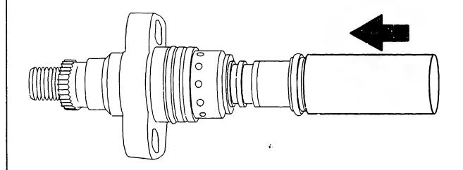
Check whether support ring (1)/ O-ring (2)/support ring (1) are correctly positioned as shown.
